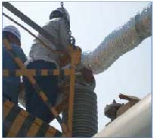
Connection set up in the Test Bushing for Transformer
