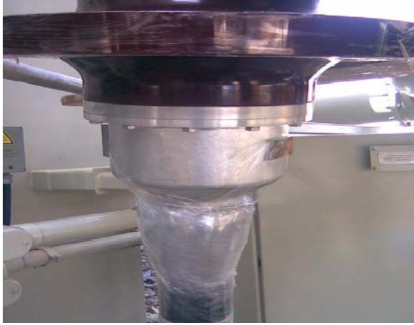
Assembled Transformer SE ready for insertion
